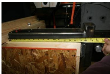
Photo 38: Alignment of Vertical Actuator
