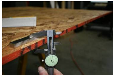
Photo 8: Thickness of OSB
