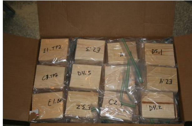
Photo 44: Specific Gravity Samples from Wall Specimens
